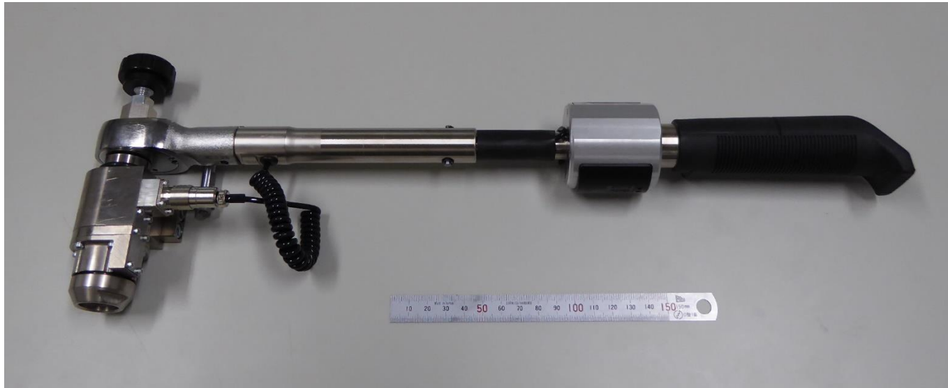
Fig. 2 Developed detection wrench of clamping force
